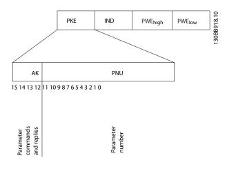
Bits no. 12-15 transfer parameter commands from master to slave and return processed slave responses to the master.
