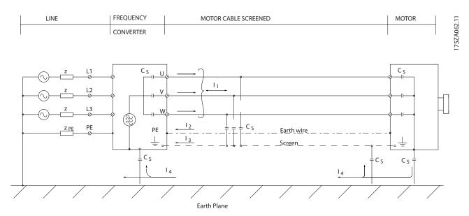
If the screen is to be placed on a mounting plate for the frequency converter, the mounting plate must be made of metal, because the screen currents have to be conveyed back to the unit. Moreover, ensure good electrical contact from the mounting plate through the mounting screws to the frequency converter chassis.
