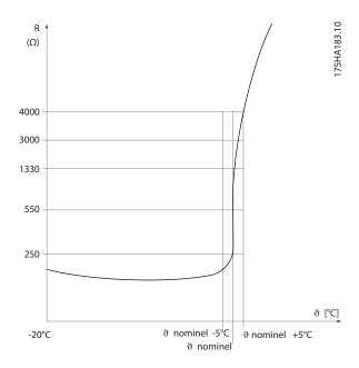
Using a digital input and 10V as power supply: Example: The frequency converter trips when the motor temperature is too high.
