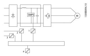
The functional galvanic isolation (a on drawing) is for the RS-485 standard bus interface.
