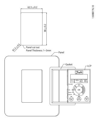
**Step 3**Place bracket on back of the LCP, then slide down.
