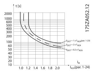
The X-axis is showing the ratio between  $I_{motor}$  and  $I_{motor}$  nominal. The Y-axis is showing the time in seconds before the ETR cuts off and trips the drive. The curves are showing the characteristic nominal speed at twice the nominal speed and at 0.2x the nominal speed.
