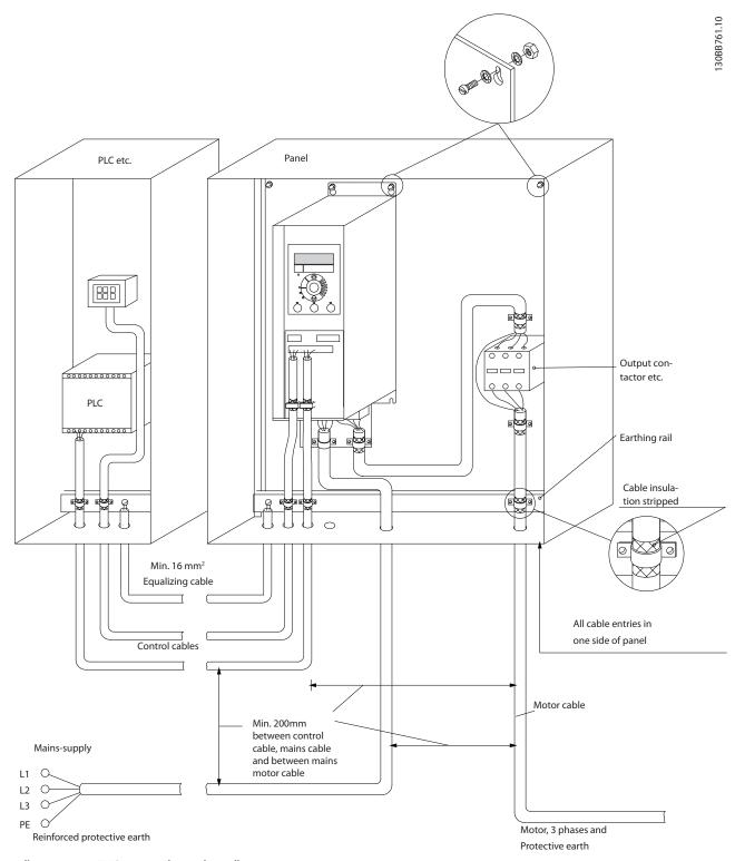
Illustration 5.1 EMC-correct Electrical Installation
