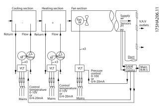
Illustration 2.6 Fan System Controlled by Frequency Converters
