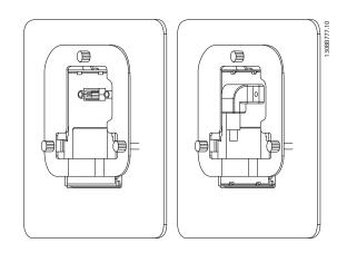
**Step 4** Connect cable to frequency converter.
